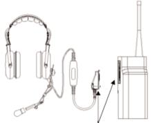
Accessory connector is attached to radio accessory jack which can be located on the side, top or bottom of a radio model. See OEM radio instruction booklet.
