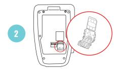
Slide the SIM card holder downward, lift the holder into an upright position and slide the SIM card into the holder. Make sure the SIM card's gold contacts face into the device and the angled corner of the card is positioned correctly (as shown in the picture on the left). Set back down the SIM card holder and slide it upwards to secure it (the SIM card should be lying flat on the device).
