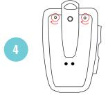
Insert the battery back into the device so that the battery contacts align and the battery label faces into the device. Then slide the battery cover back into place and screw it shut. Do not over tighten.
