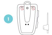
Turn off the device. Open the battery cover with the provided screwdriver and remove the device's battery.
