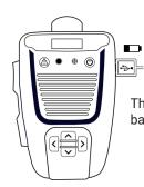
The display will show the battery level for 30 seconds.
