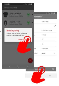
To unpair your device, press it for long in the menu and accept the unpairing request OR go the device details menu and press the "REMOVE DEVICE" button.
