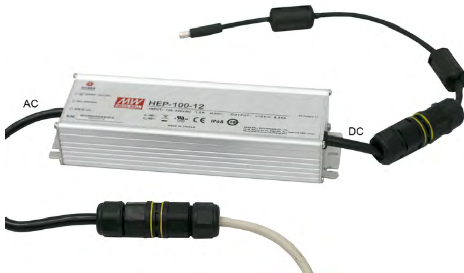
Figure 44: Assembled SLR 1000 Repeater Power Supply
