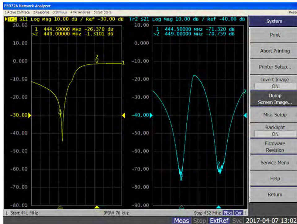
Figure 27: Rejection of Each Port for UHF Duplexer
