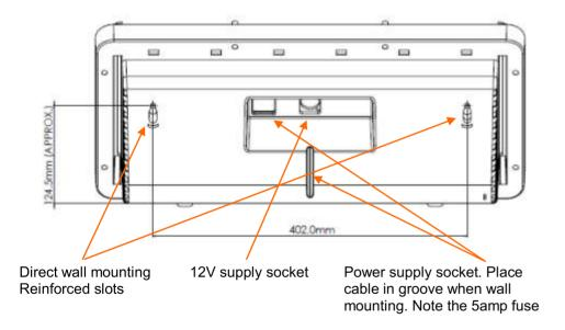
This 12 way charging unit occupies a footprint very similar to that of a standard competitive 6 way charger. The unit can be desk or wall mounted. No further unit fixings are required for wall mounting. There are 2 points for screw fixings. We can accept no responsibility for the type of fixings or the surface used for wall mounting. Or the stability of the unit when secured in position. Wall mounting is entirely at the user's risk.
