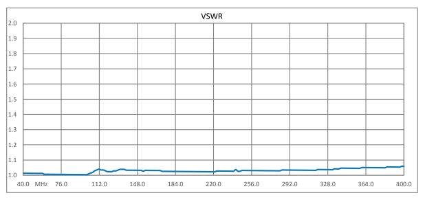
Click the following link (or enter part number in "SEARCH" on website) to obtain additional part information including price, inventory and certifications: Type N F/F Coaxial RF Surge Protector, 40MHz - 400MHz, 100W, IP67, 60 V Max., 2.5mJ, 20kA, Hybrid, Bracket Down, Hole Mount BGXZ-60NFNF-ALT
