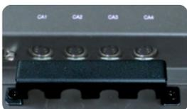
Fix the bracket jack with provided screws after connecting the cameras.
